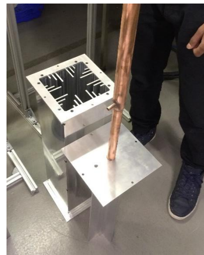
Fig. 1. Heat pipe and PCM unit.
