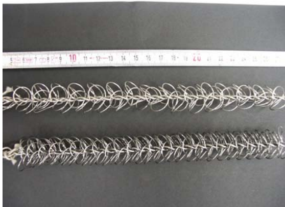
Fig.1: High and low density turbulence promoters (hiTRAN)
